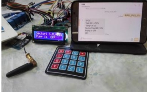
Fig. 9 Response of the SPCS system to the user SMS '$SND_SPCS_ST/'.
