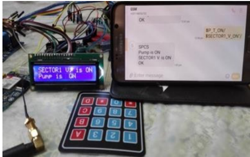
Fig. 10 Response of the SPCS system due to user SMS '$P_T_ON' and '$SECTOR1_V_ON'
