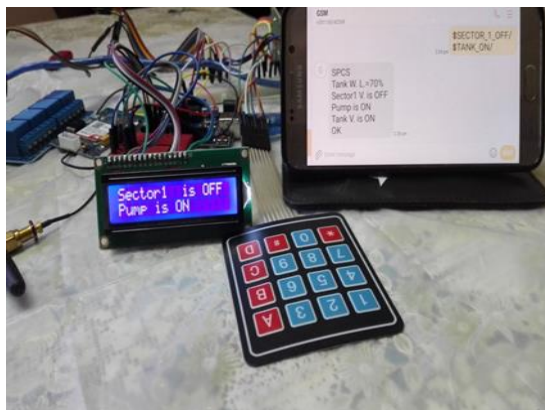
Fig. 10 Response of the SPCS system due to user SMS '$P_T_ON' and '$SECTOR1_V_ON'
